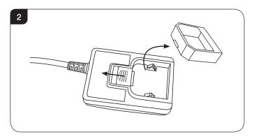
1.4 Slide back the catch and insert the required plug, ensuring that both tabs engage to hold the plug securely, see Diagram 3.
