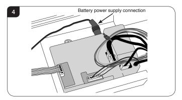
Secure the battery cable in the appliance so it may be used again in case of power failure.
