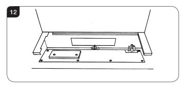
7.4 Isolate the gas supply at the isolation device and disconnect the gas inlet, see Diagram 13.
