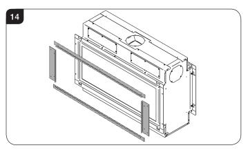
5.2 Fix foam seal to the rear of the outer flange of the appliance, see Diagram 15.
