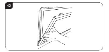
12.4 Manoeuvre the frame up towards the left side to locate the left hinge pin.
