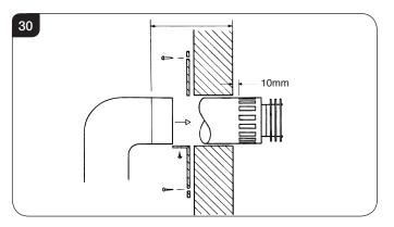
A wall plate is supplied to fix the flue to the wall:
