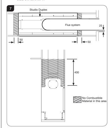
3.2 DO NOT PACK THE VOID AROUND OR ABOVE THE APPLIANCE WITH INSULATION MATERIALS SUCH AS MINERAL WOOL.
