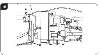
7.8 Disconnect the battery extension lead, Diagram 16, B.
