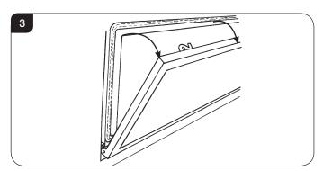
3.5 Remove the securing spring clip from the bottom-right of the window frame, see Diagram 4.
