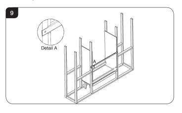
4.7 Fit the support bar into the studwork at the correct height, see Diagram 10.
