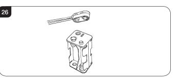
7.3 Correctly position the four new AA size batteries and re-assemble the battery holder as shown, see Diagram 27.
