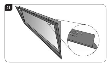
5.19 If the Edge+ is too loose the tabs can be bent up to gain better purchase on the edge of the appliance box.If the Edge+ is too tight the tabs can be bent downwards to give more clearance.
