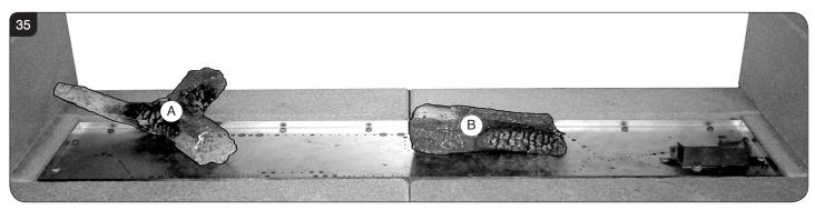
11.3 Use all the vermiculite to fill the burner tray between Logs A and B. Spread evenly across between the logs, so the whole burner is covered, see Diagram 36.
