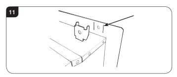
4.9 Fix foam seal to the rear of the outer flange of the appliance, see Diagram 12.
