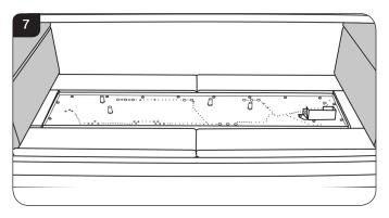
5.3 Remove the lower liners around the burner tray, see Diagram 8.
