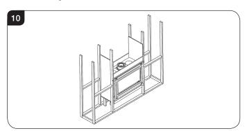
4.8 Attach the 4 x frame fixing brackets to the appliance, see Diagram 11.
