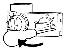
Disconnect the end of the ignition lead from the valve body, see Arrow B, note the existing route of the ignition lead.
