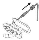
Undo the thermocouple from the back of the gas valve.
