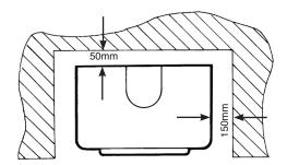
In a non-combustible recess be careful to allow enough clearance at the sides and rear of the appliance to perform spillage tests and reach the controls.
