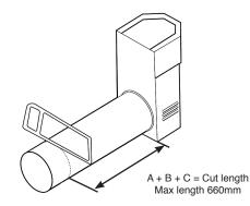
Measure the total wall thickness to give Dimension C. Add Dimensions A+B+C to give the total required length of the flue pipe. This will give the correct engagement to the appliance spigot and maintain the minimum distance between the appliance and the internal wall.
