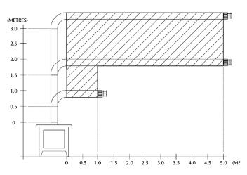
This kit provides the minimum materials. Extra lengths can be added to the vertical and horizontal sections.
