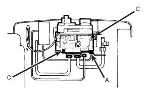
Remove the control valve cover and disconnect the ignition lead from the gas valve.
