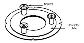
Remove the restrictor plate that is current in place and fit the 47mm  $\varnothing$  one from the kit.
