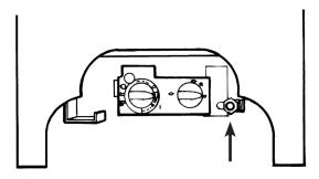
Connect a suitable pressure gauge to the test point located on the inlet fitting and turn the gas supply on. Light the appliance and check all gas joints for possible leaks. Turn the appliance to maximum and check that the supply pressure is as stated on the databadge. Turn the gas off and replace the test point screw, turn the gas on and check the test point for leaks.
