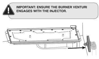
NOTE: Before replacing the burner, make sure the silicone seal around the injector is intact.
