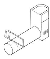
Terminal dimensions: 395 x 200 x 200 mm (H x W x D) Guard supplied Cut to length as required on site.
