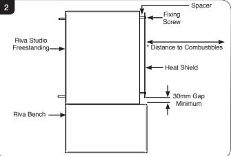
1.2 Take care to not over tighten the fixing screws it using a power screwdriver.
