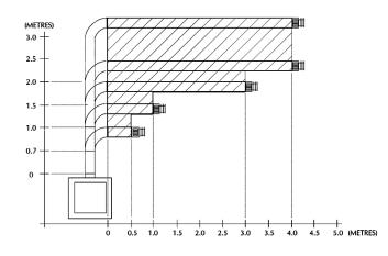
Start of bend to centre line of horizontal flue 170mm. Centre line of vertical flue to end of bend 220mm.
