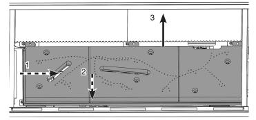
Carefully remove through the front of the appliance. Place carefully to one side.
