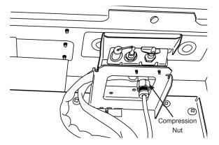
Remove the Ignition Lead from the Electrode.
