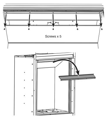
The baffle can now be removed by lowering the front edge and pulling forward through the front of the appliance. TAKE CARE NOT TO DAMAGE THE SIDE PANELS.
