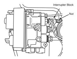
Unplug the Ignition Lead from the Control Box.
