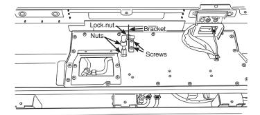
Remove the 2 screws and the bracket.
