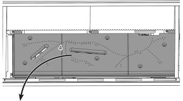
The gas supply enters through the silicone panel located on the left-hand side on the rear of the outer box; this will need to be slit with a sharp knife prior to passing the supply pipe through.
