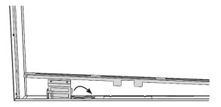
Remove the screws at the base of the glass frame see A.
