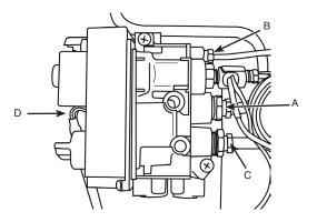
Remove the Thermocouple from the Interrupter Block.
