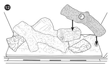
The back edge of log F should rest against the back liner.
