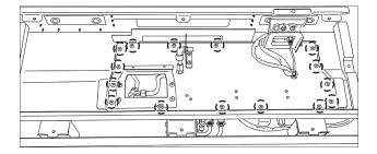
Lift the back of the control assembly and tilt forward to enable access to the controls.
