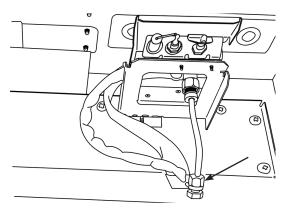
Feed Ignition Lead and Thermocouple complete with Vidaflex through metal plate.
