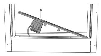
Disconnect the battery lead from the battery pack.
