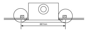
This diagram shows the minimum clearance position when installing the appliance into studwork - it is vital to ensure the opening is wide enough to accommodate the fixings for the front.
