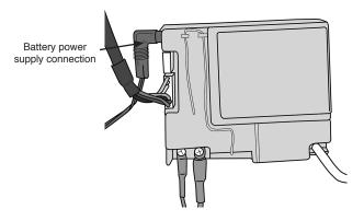
The Control Assembly can now be lifted and removed through the front of the appliance.
