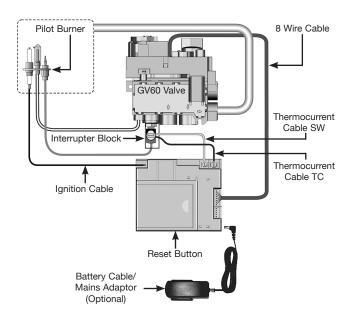
After replacing the control box you may need to reprogram the handset.
