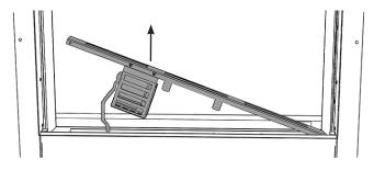
Disconnect the battery lead from the battery pack attached to the lower slotted trim.
