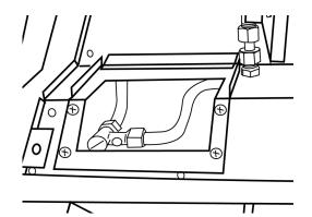
Remove the 15 screws securing the control assembly.
