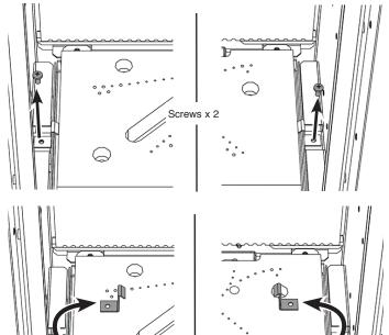
Slide the burner unit to the right, pull slightly forward and lift from the back.
