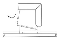
Remove the cover by sliding off in the direction of the arrow as shown.
