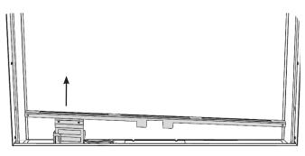
Disconnect the battery lead from the battery pack attached to the lower slotted trim.
