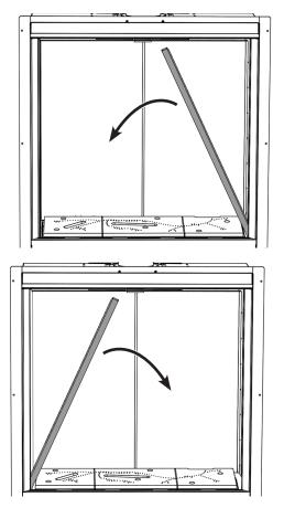
The Side Liners support the 2 piece Back Liner. Ensure the back liners are supported when the sides are removed.
