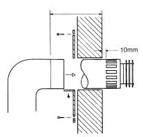
A wall plate is supplied to fix the flue to the wall:
