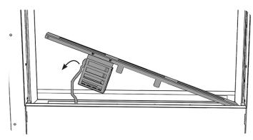
Remove the screws at the base of the glass frame, see A.
