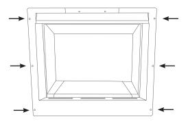
Build the chimney breast up to coincide with the edge, allowing for the front to be skimmed level.
