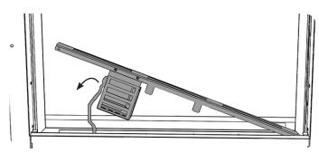
Remove the screws at the base of the glass frame see A.
