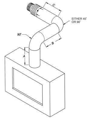
When A = 1.5 to 1.999 metres B + C = 2.0 metres maximum When A = 2 metres to 3 metres B + C = 3 metres maximum
