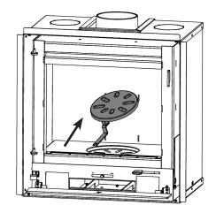
To remove the Main Grate, lift from inside the grate cutout and rotate out to clear the firebox.
