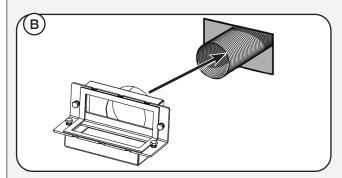
Pull the Outdoor Air Adapter forward through the cut out from behind the fire box.
