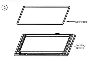
Squeeze a generous bead of fresh Stovax Thermic Seal glue into the rope locating groove.
