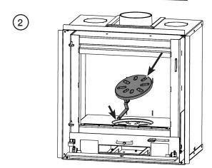
NOTE: When refitting, ensure the Centre Grate Arm lines up with the Primary Air Control Pin.
