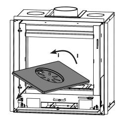
Ensure that the seal tape on the underside of the grate  $(20 \times 2 \text{ mm})$  and log guard  $(10 \times 2 \text{ mm})$  is in good condition and correctly fitted. If not, replace with new.
