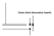
125mm hearth thickness (Constructional and Decorative combined) If installed at a height above 200mm from the floor there is no need for a constructional hearth in front of the appliance.
