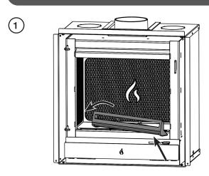
Secure the Log Guard in place using the 2 x Hex Socket M5 screws.
