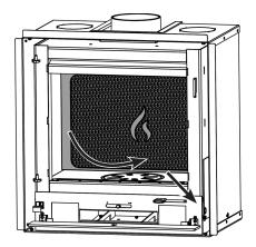
Do not operate with the firebricks removed.
