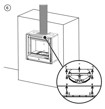
Remove bar once the flue has been secured.
