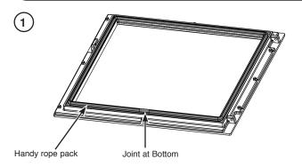
To maintain the safe use of the appliance damaged or worn door sealing rope must be replaced.
