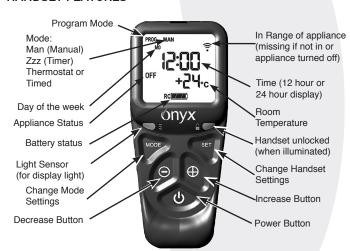
The Icon at the bottom of the screen displays the battery condition of both the batteries in the handset and in the Control Box alternatively.
