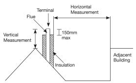
The datum for vertical measurement is the point of discharge of the flue from either the point of discharge of the flue or 150mm above insulation, whichever is the lower.
