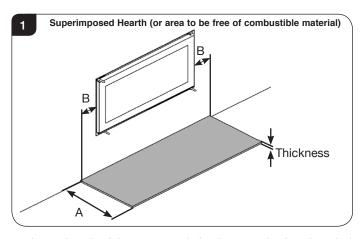
3.2 If this appliance is installed in an elevated setting it is recommended to increase the front hearth depth to safely contain any falling logs or embers. The higher the appliance is installed the deeper the hearth should be to avoid scorched floor coverings.
