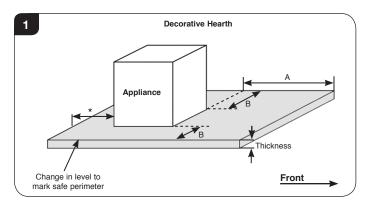
3.2 If this appliance is installed in an elevated setting it is recommended to increase the front hearth depth to safely contain any falling logs or embers. The higher the appliance is installed the deeper the hearth should be to avoid scorched floor coverings.
