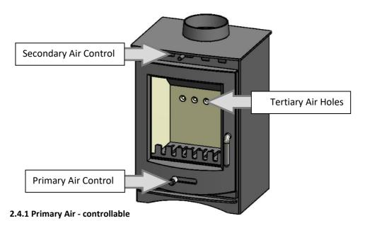
Primary air is controlled via the sliding vent in the bottom of the door. This provides an air draught through the grate to the bed of the fire. Slide right to open and left to close. Open this when you start a fire, and to regulate solid fuels other than wood. It should be closed when a wood fire is established for the best efficiency but can be used to give a wood fire a boost when it is dying out.
