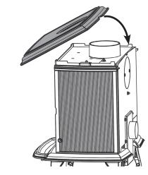
Seal the connecting joints.
