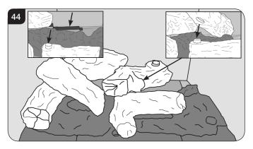
9.8 Sit the first hole in the bottom of the left hand side of Log M on the stud of Log H and secure by fitting the middle hole on the right hand side over the stud in the fuel bed by the burner port, see Diagram 45.
