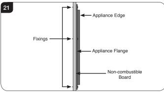
6a.10 Fit non-combustible board to the board around the appliance, see Diagram 22. Ensure distances to combustibles are observed, see Diagram 16.
