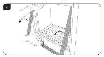
3.6 Undo the screws to remove the left hand metal side cover see Diagram 8.
