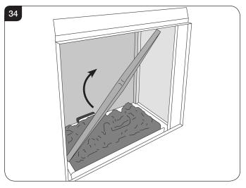
8.7 To fit the Right Hand liner insert through the front of the appliance tilting the top inwards towards the centre of the firebox before lowering into position, see Diagram 35.
