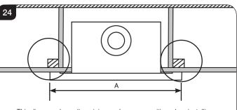
This diagram shows the minimum clearance position when installing the appliance into studwork - it is vital to ensure the batterning is wide enough to accommodate the fixings for the front.
