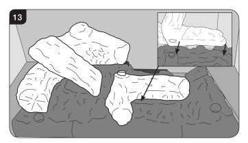
5.7 Rest Log J on the raised stud on Log H. The rear of the effect should rest on the metal bracket at the back of the burner tray, see Diagram 14.
