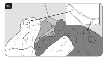
5.9 Log M should rest on the flat plain behind the stud for the Log arrangement to be complete, see Diagram 16.
