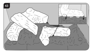
9.7 Rest Log J on the raised stud on Log H. The rear of the effect should rest on the metal bracket at the back of the burner tray, see Diagram 44.
