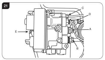
7.8 Remove the 2 screws securing the valve to the support bracket and withdraw the valve.
