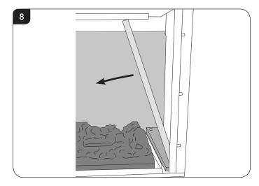
3.7 To remove the Left Hand liner first tilt inwards towards the centre of the firebox before lifting up and pulling out through the front of the firebox, see Diagram 8.
