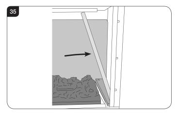
8.8 To fit the Left Hand liner insert through the front of the appliance tilting the top inwards towards the centre of the firebox before lowering into position, see Diagram 35.
