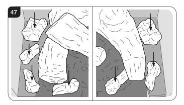
9.11 Lay Embaglow over the small ports in the base of the burner tray. This will create a glowing effect when the appliance is lit, see Diagram 48.
