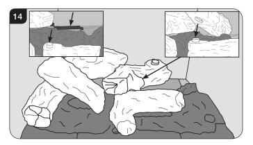
5.8 Sit the first hole in the bottom of the left hand side of Log M on the stud of Log H and secure by fitting the middle hole on the right hand side over the stud in the fuel bed by the burner port, see Diagram 15.
