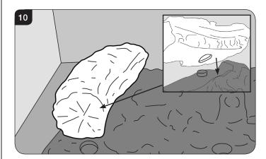
5.4 Place Log L behind the Log A on the flat plain and locate the rear of the log on the metal bracket. The log should rest between the lip of the bracket and the rear liner, see Diagram 11.
