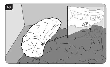
9.4 Place Log L behind the Log A on the flat plain and locate the rear of the log on the metal bracket. The log should rest between the lip of the bracket and the rear liner, see Diagram 41.
