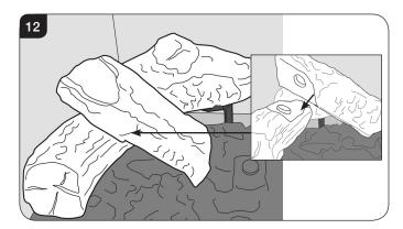
5.6 Place Log H on the centre of the burner tray. There is a raised stud in the fuel bed which securely locates the log in place. The right hand side rests on the raised section at the end of the air cutout, see Diagram 13.
