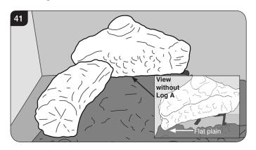
9.5 Place Log G on top of Log A. There is a hole on the underside of Log G which fits over the raised stud on Log A to secure in place. The end of the log sits on the raised section of the burner tray, see Diagram 42.
