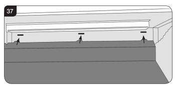
8.11 Replace the 3 screws to secure it to the roof of the firebox, See Diagram 38.
