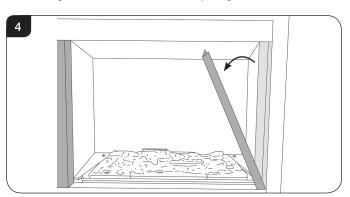
3.2 Lift out the bottom slotted trim, see Diagram 5.
