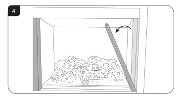
4.4 Lift out the bottom slotted trim, see Diagram 5.
