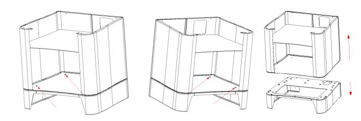
Feed the mains cable through the cut out in the legs then place the stove engine onto the legs and secure via the two screws on the under side of the feet and two on the rear on the stove engine.
