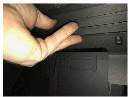
To remove rear steel baffle is Simply push this away from the holding frame, which it rests on, and twist it to fit through the opening.
