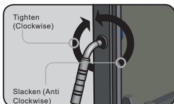
Insert the supplied Allen key into the hole in the side of the door containing the set-screw. Turn it anti-clockwise to slacken the set-screw until the door handle becomes loose. Once loose, turn the handle the correct way as shown in the drawing to the left. On completion, slowly re-tighten the set-screw until the handle is set properly and the door shuts tightly again.
