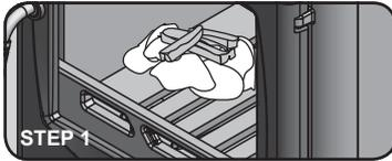
**Step 1** Place rolled up crumpled paper at the back of the appliance. Next, place a small amount of tinder/kindling on top of the paper followed by a few larger pieces of wood. Light the paper and close the door. NEVER USE FLAMMABLE LIQUIDS
