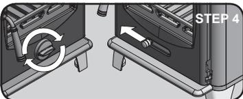
**Step 4** Once the fire is established, both air controls can be reduced in order to maintain a steady burn rate dependant on your fuel type. On the SP model, turn the spinner clockwise to close. On the SL model, push the slider to the left to close. Push the top air intake to the right.
