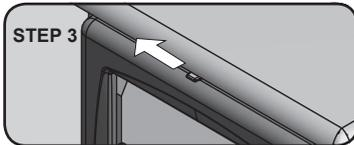
**Step 3** Allow the fire to burn until all the pieces of wood are alight and burning. The top air intake (Secondary air) can be used if additional air is needed. Push the slider to the left to open. More larger pieces of fuel can now be added. Be careful not to add so much fuel that it is in danger of overflowing the fuel bar or touching the glass.
