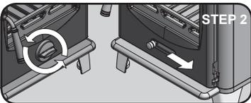
**Step 2** Open the front air control (Primary air) fully, using the glove provided. On the SP model, turn the spinner anti-clockwise to open. On the SL model, push the slider to the right to open.
